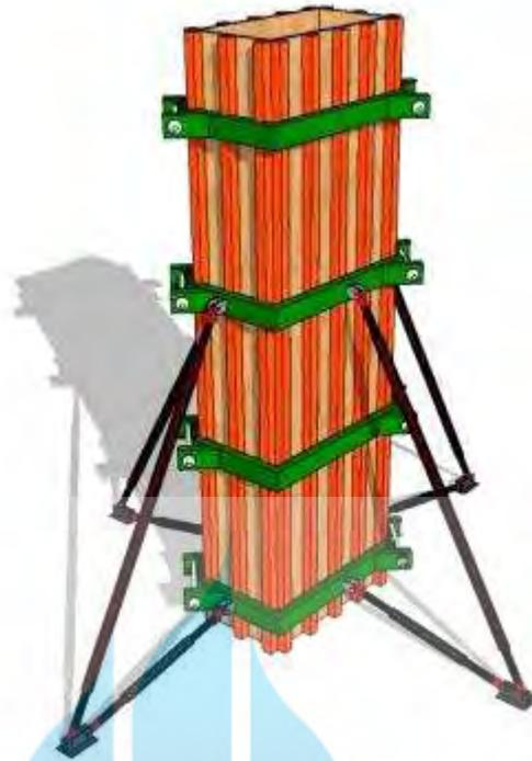
Gambar 5.3 Pemasangan Pipa Support
