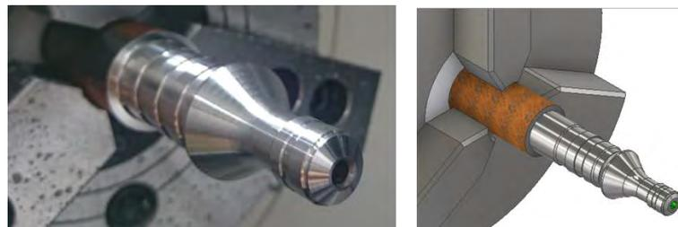
Gambar 4.29 Proses *Drill Diameter* 4 mm
