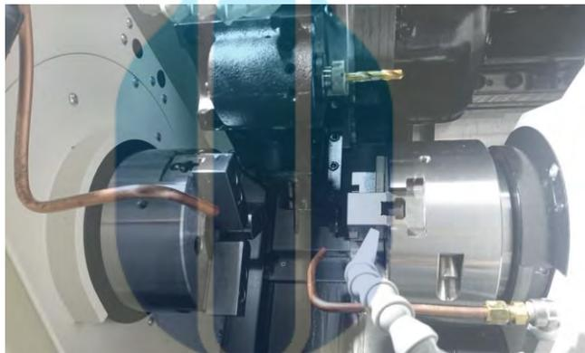
Gambar 4.33 Proses *Transfer & Cut Off*
