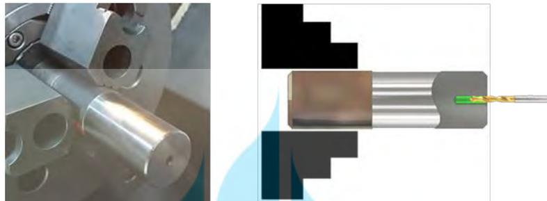
Gambar 4.7 Proses *drilling* diameter 4
