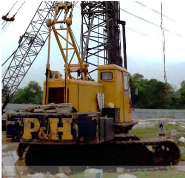
Gambar 5.4 Alat Pancang Diesel Hammer
