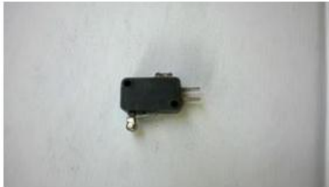
Gambar 6. Saklar switch power window
