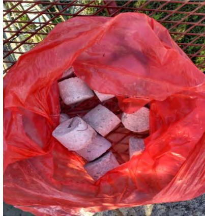
Gambar 4.4. Beton Decking
