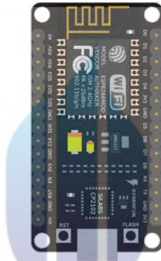
Gambar 2. 2 Versi nodemcu esp8266 1.0
