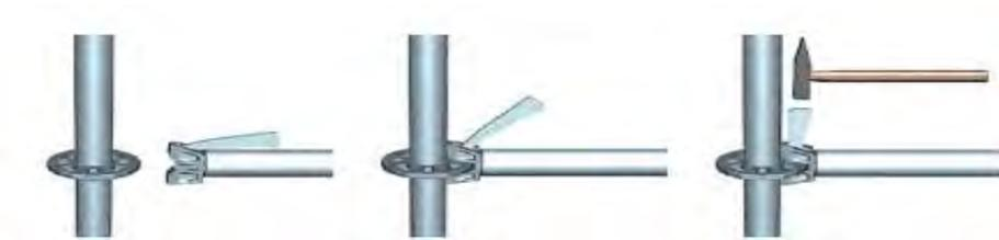
**Gambar 2. 2 *Ring-lock Modular System***
