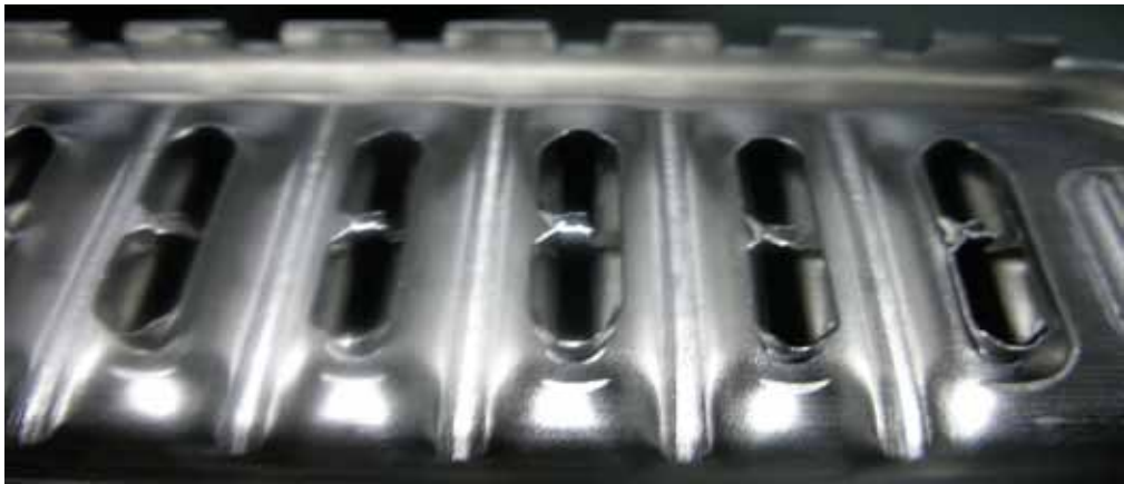
Gambar : 3.2. Hasil Proses Expand
