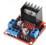
Gambar 2.8 Driver Motor MDL298N
