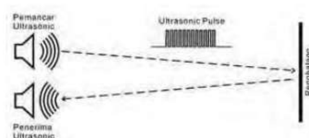
Gambar 2. 5 Prinsip kerja sensor ultrasonic
