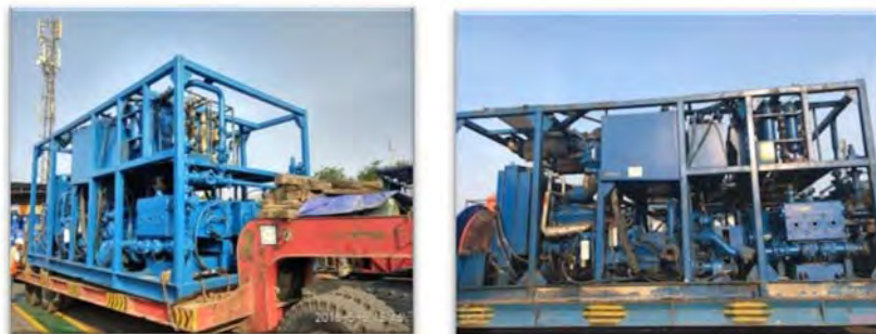
Gambar 4.5. Twin Pompa HT-400
