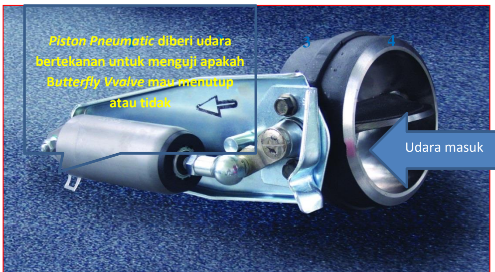
Gambar 4.14 Exhaust Brake Valve leakage test
