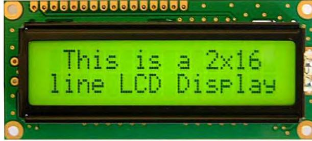
Gambar 2.12 *interface* Modul LCD 2 x 16
