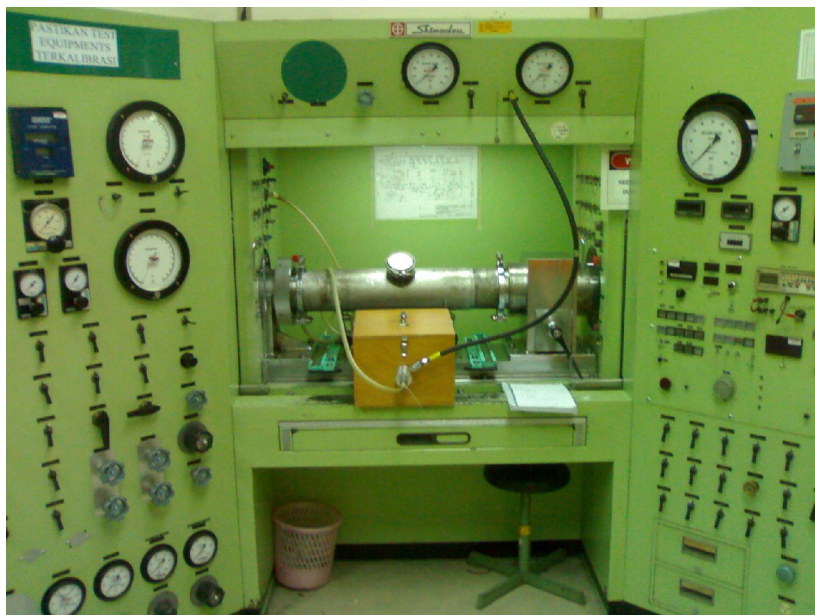
( Proses pengetesan Pompa Vakum ) ( Sumber : GMF Aero Asia, Pneumatic Shop )
