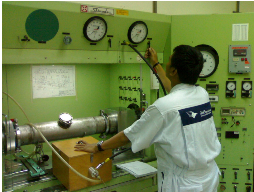
( Proses pengetesan Pompa Vakum ) ( Sumber : GMF Aero Asia, Pneumatic Shop )
